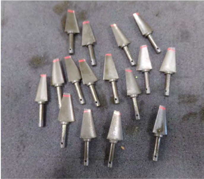
17) Driven Compressor IGV
