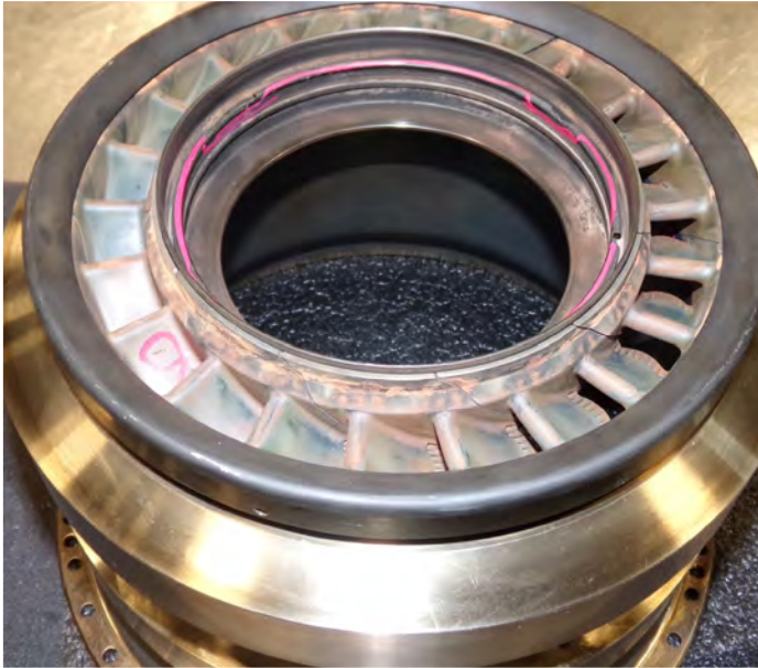
21) 1st Stage Turbine Stator Assy
