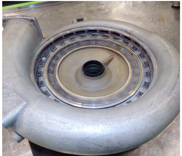
8) Driven Compressor Bearing Housing
